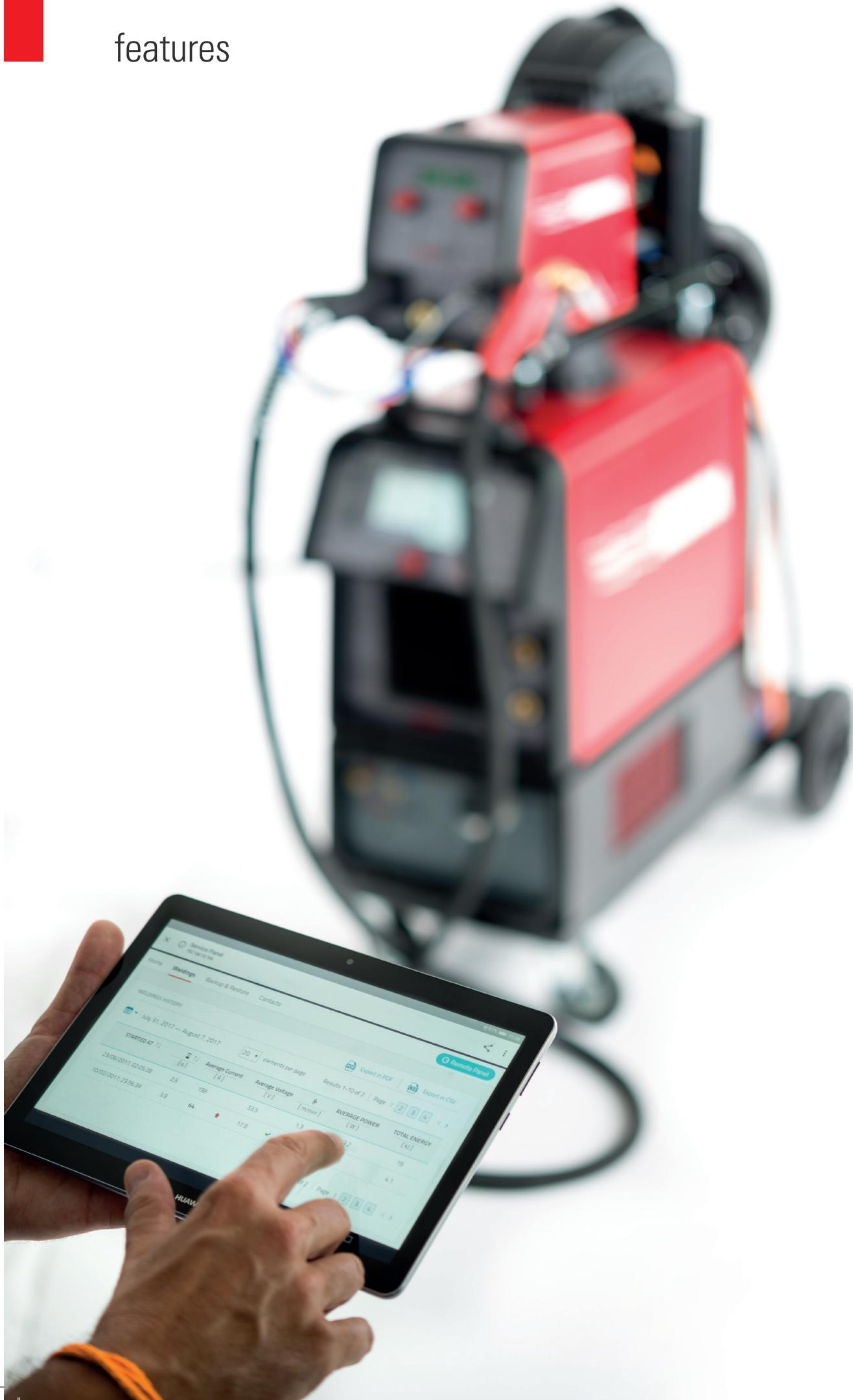
Compact and lightweight wire feed unit with two 7-segment display and user friendly operator controls. In addition to the MIG/MAG Euro torch connection, there is also a devoted connection for a standard TIG torch.
